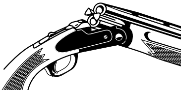
Break Action: shells are manually inserted into chamber and may be ejected manually or automatically depending on the model.
